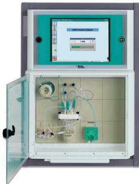
2035 Process Analyzer for potentiometric titration measurements
