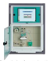
2035 Process Analyzer for potentiometric titration measurements
